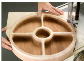
Bandsaw the exterior to final shape.
